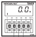
Dip switches for time setup (001 ~ 999)
