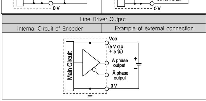
\* The output circuit of A, B, Z phase (Line drive output A,  $\bar{A}$ , B,  $\bar{B}$ , Z,  $\bar{Z}$  phase) is same.
