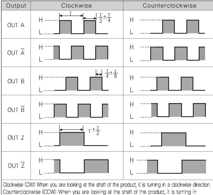
Clockwise (CW): When you are looking at the shaft of the product, it is turning in a clockwise direction.
